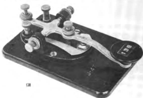
● (176) Key used by U.S. Military in WW-II. No markings. Nicknamed "The Pressure-cooker" by Elwood's XYL/Edith. Small key mounted in flame-proof compartment. Heavy construction.
